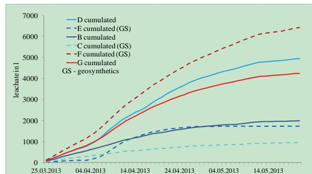
Fig 3. Cumulated leachate in different sections (M1- red, M2 - blue) period from end of March to the first filling
