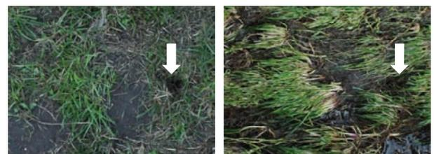
**Fig 23.** Detail cross section D, a) Initial situation (bare areas and vole hole) b) 4th overtopping
