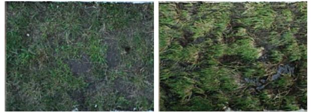
**Fig 12.** Cross section D (52 x 38 cm), flume 1, section 6, a) Initial situation b) After 4<sup>th</sup> overtopping
