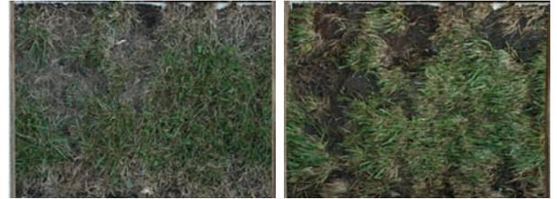
**Fig 13.** Cross section E (52 x 38 cm) with erosion mat, flume 1, section 6, a) Initial situation b) After 4<sup>th</sup> overtopping
