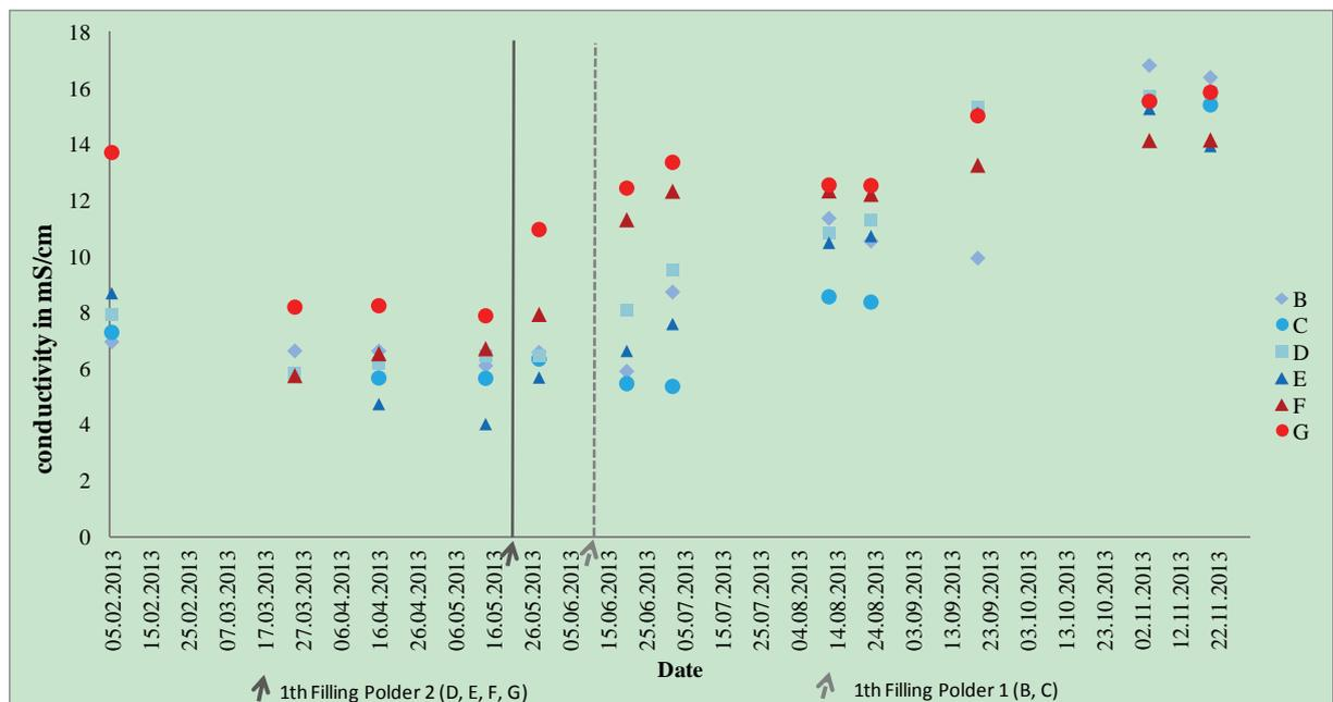
**Fig 4.** Conductivity in leachate from different cross sections (material M1 – red marks, material M2 – blue marks)
