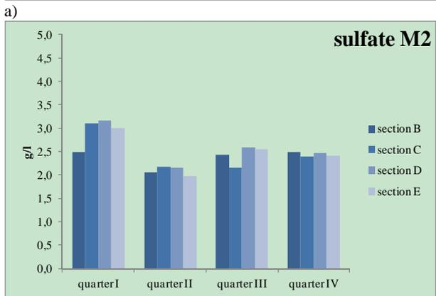
Fig 6. Content of sulfate in leachate a) material M1 b) M2
