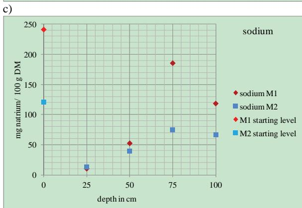
Fig 2. a) to d) Content of salt ions in the different layers of the compaction testing field (M1 and M2)
