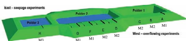
**Fig 1.** Rostock test dike with different cross-sections and applied materials
