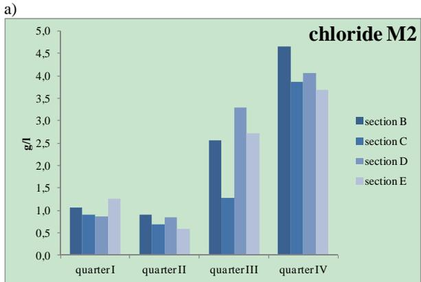
Fig 5. Content of chloride in leachate a) material M1 b) M2
