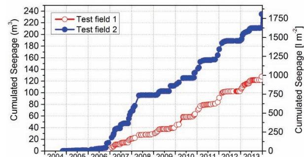
**Fig 5.** Cumulative seepage of both test fields
