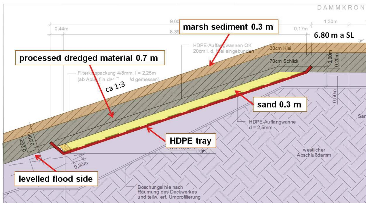
**Fig 3.** Vertical cut through test field 2
