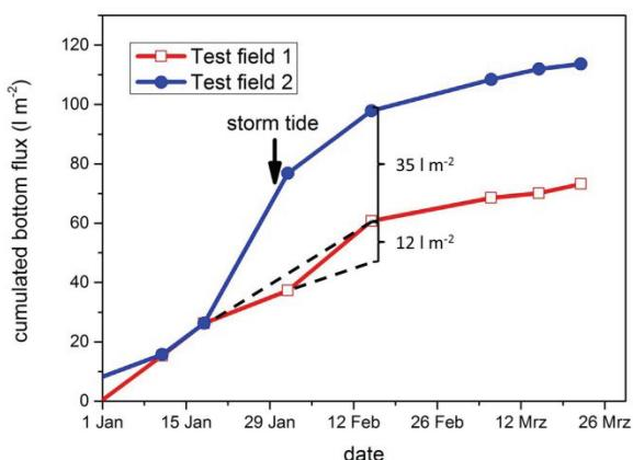
**Fig 7.** Bottom flux of both test fields at storm tide 31.1.2013 (arrow)
