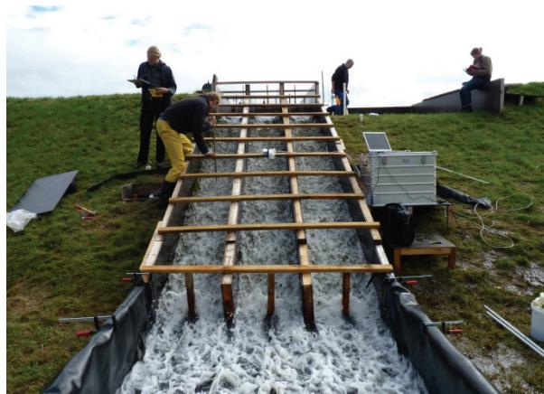
**Fig. 10.** Experimental procedure cross-section H, first discharge stage ( $q \approx 0.05 \text{ m}^3(\text{m}\cdot\text{s})^{-1}$ ,  $v \approx 1.57 \text{ ms}^{-1}$ ,  $\tau \approx 270 \text{ Pa}$ ), measurement of flow velocity in the left flume
