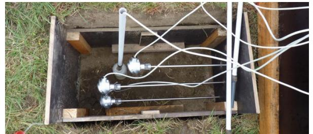
**Fig. 9.** TDR-sensors and tensiometers under the flumes
