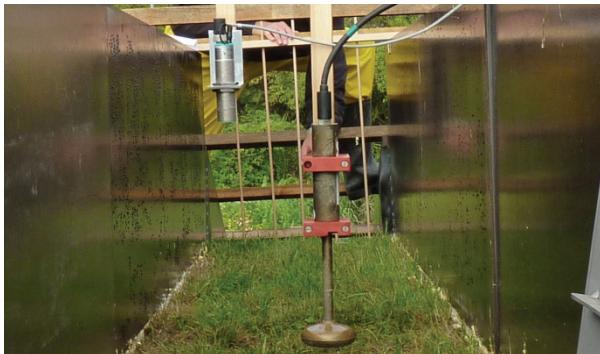
**Fig. 7.** Ultrasonic sensor to measure runoff depth (left), magnetic-inductive sensor to measure flow velocity (right)
