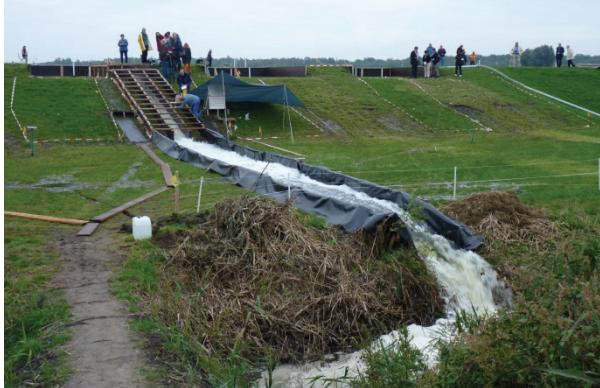
**Fig. 6.** Runoff channel to lead the water back to the basin
