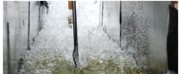
**Fig. 15.** Flow velocity measurement, turbulent conditions with a lot of air entrainment
