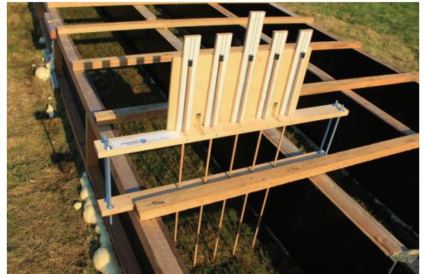
**Fig. 8.** Pin profiler to measure the soil loss/ gain and the discharge depth
