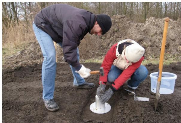
**Fig 4.** Sampling of installed dredging spoil
