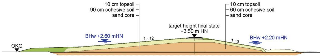
Fig 1. Standard cross-section of the East Zingst dike
