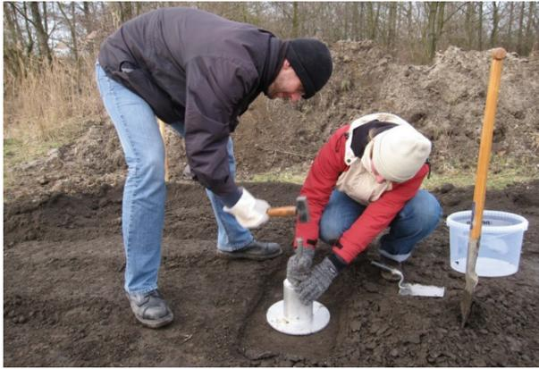
Fig 4. Sampling of installed dredging spoil
