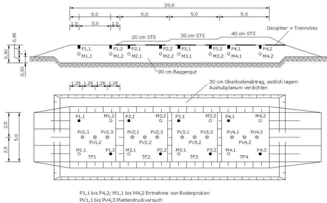
**Fig 3.** Structure of test area and location of sampling point and load plate tests [U 2]
