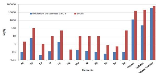
**Fig 8.** Leaching results on core material after 60 days (blue) compared to the limit (red) expressed in mg/kg
