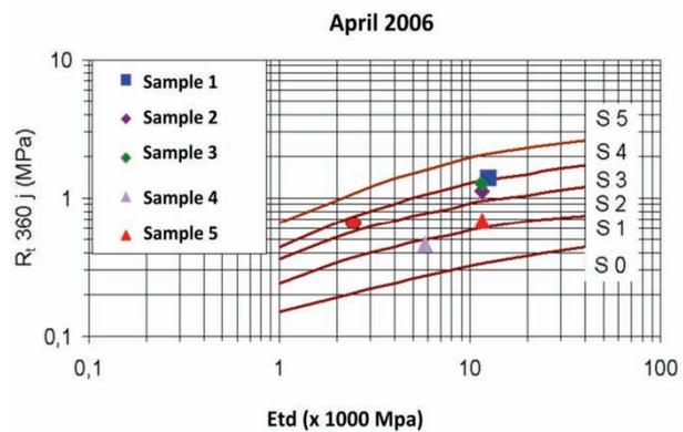
**Fig 6.** Direct tensile strength ( $R_t$  in MPa) versus the Elastic modulus ( $E_{td}$  in GPa) results of the lab scale results and of the cores of the 2005 pilot test road (red dot)
