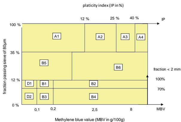
**Fig 1.** French standard NF P 11-300: classification of materials used in the construction of embankments and subgrade road infrastructure.
