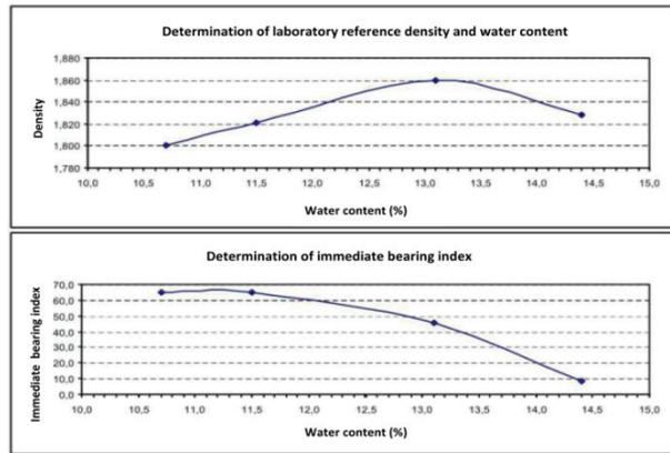
**Fig 5.** Proctor curve and IPI-curve of sediment after treatment
