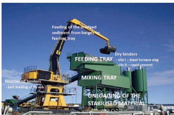
**Fig 7.** The principle of process stabilisation
