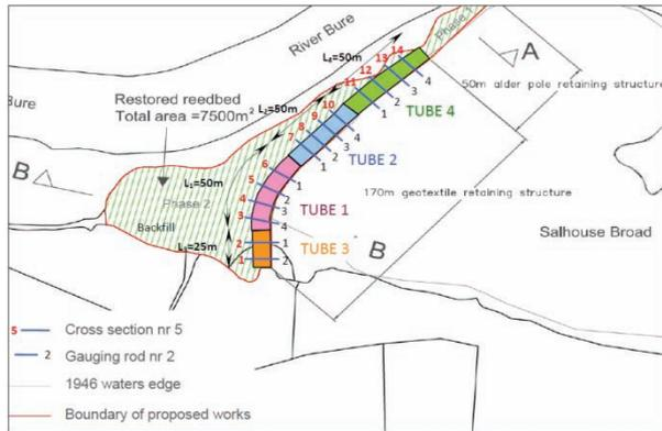
**Fig 9.** Schematisation of the geotextile tubes and cross sections.
