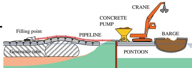
**Fig 7.** Schematisation of the execution phase (not to scale).
