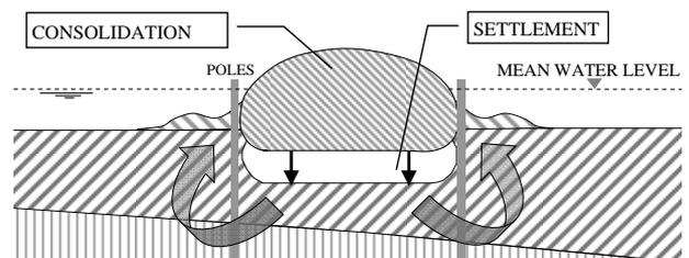
**Fig 4.** Consolidation and settlement of the geotextile tubes.
