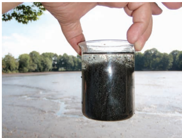
Fig 9. Sludge after addition of chitin based flocculant for soil improvement
