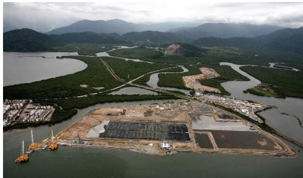
**Fig 11.** Tube dewatering site, completed and started with overburden placement early 2012
