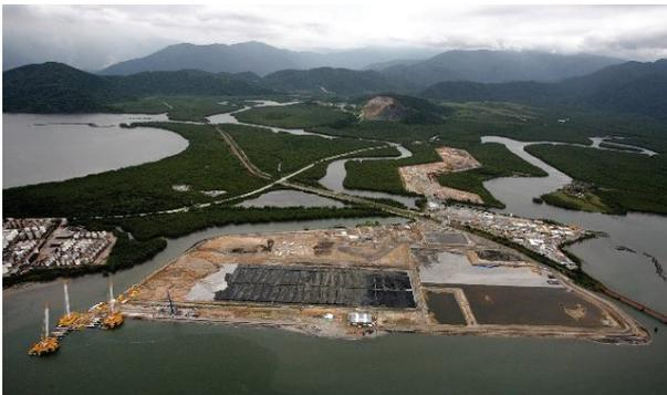
**Fig 11.** Tube dewatering site, completed and started with overburden placement early 2012
