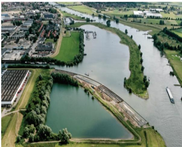
**Fig 4.** Geotextile tubes in place
