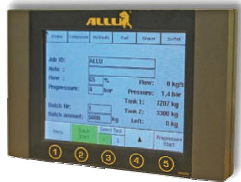
**Fig 7.** DAC control panel
