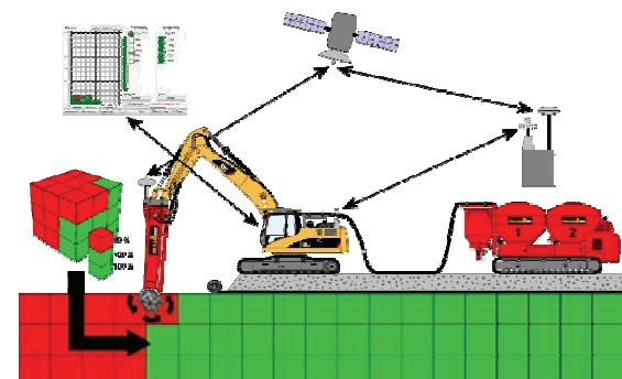
**Fig 8.** 3D positioning system
