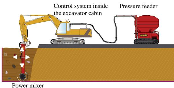
Fig 2. In-situ mixing process
