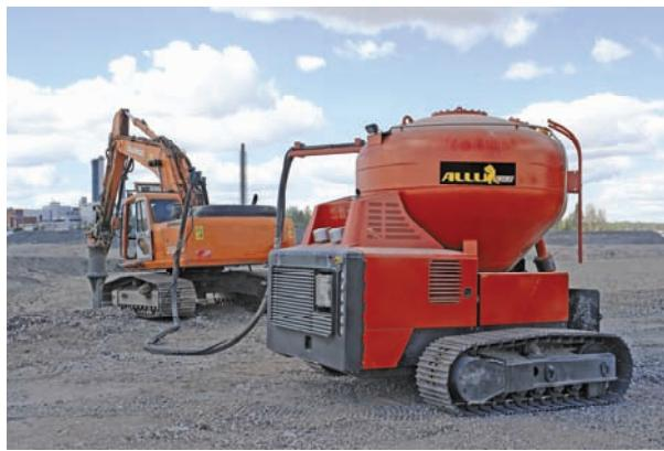
**Fig 5.** Pressure feeder with one binder tank
