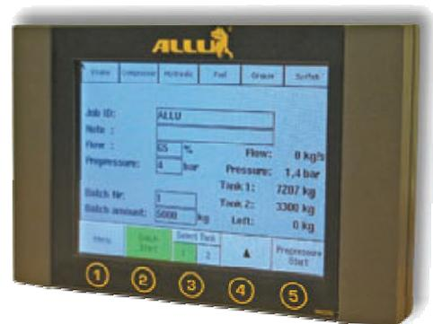
Fig 7. DAC control panel
