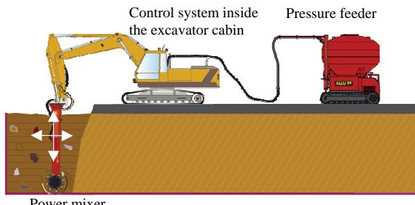
**Fig 2.** In-situ mixing process
