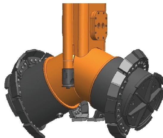
**Fig 4.** Mixing head with replaceable blades and binder feeding nozzle
