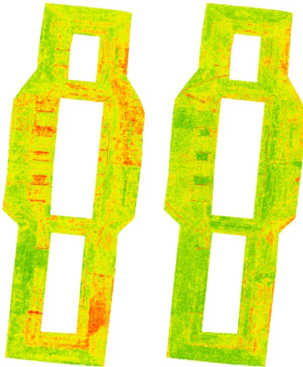
Figure All.64. Comparison of cover ratio of the test dike after winter season in April (l) and mid-June (r) 2013 (aerial images from [42])
