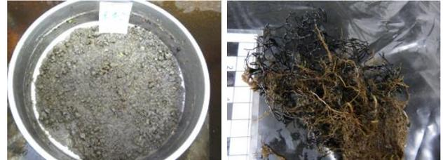
Figure All.53. a) Soil and stones, rests of roots and organic material in the sieve, b) Washed out root system with rooted RECP
