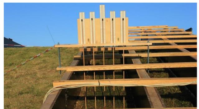
Figure All.18. Pin profiler to measure the soil loss/ gain and the discharge depth
