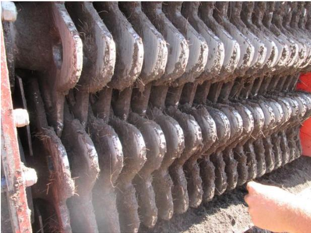
Figure All.140. Drums of the screener bucket for fine screening
