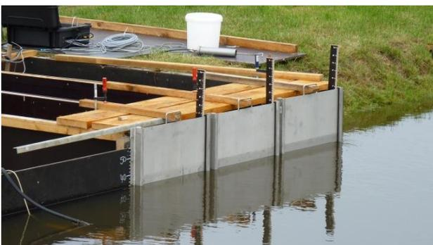
Figure All.15. Closed water inlets at cross-section H
