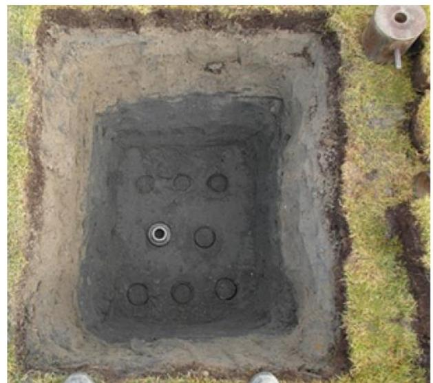
Figure All.79. Obtaining undisturbed samples of bottom ash-dredged sand mixture from the excavation at the test dike in Gdańsk.
