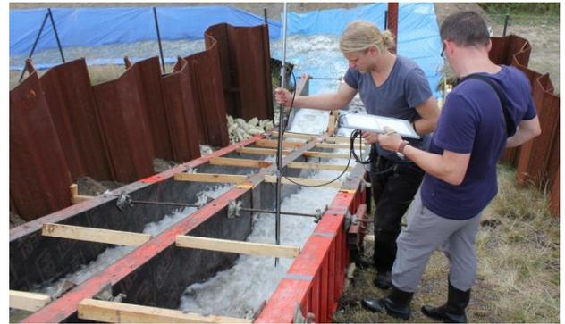
Figure All.98. Runoff channel to lead the water back to the Vistula
