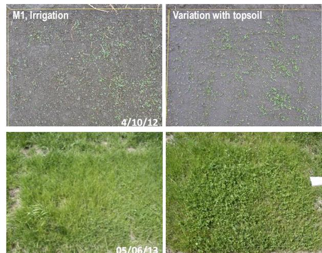
Figure All.63. Two different variations of the seeding test on the dike embankment – compacted surface, M1 with initial irrigation (l) and variation with topsoil (2 cm) above M2 (r)
