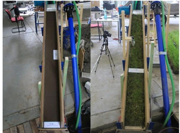
Figure All.5. Installed samples, unvegetated (l) and vegetated (r)
