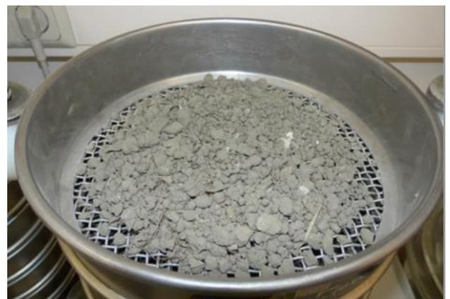
Figure All.143. Dried fibre and soil mixture during sieving
