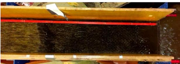
Figure AII.7. Downstream erosion above the geomat (GMA), originate at a crosswise crack (M2, December 2013)
