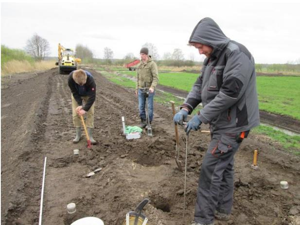
Figure All.129. Compaction control in the cover layer made of dredged material 04-2014
