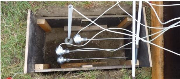
Figure All.19. TDR-sensors and tensiometers under the flumes
