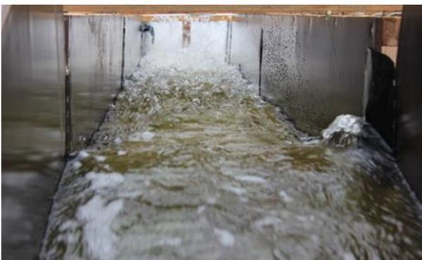
Figure All.25. Turbulent flow conditions in with air entrainment in the lower parts of the flume
