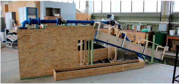
Figure All.3. Laboratory flume, sample boxes in the front
