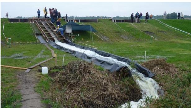
Figure All.16. Runoff channel to lead the water back to the basin
