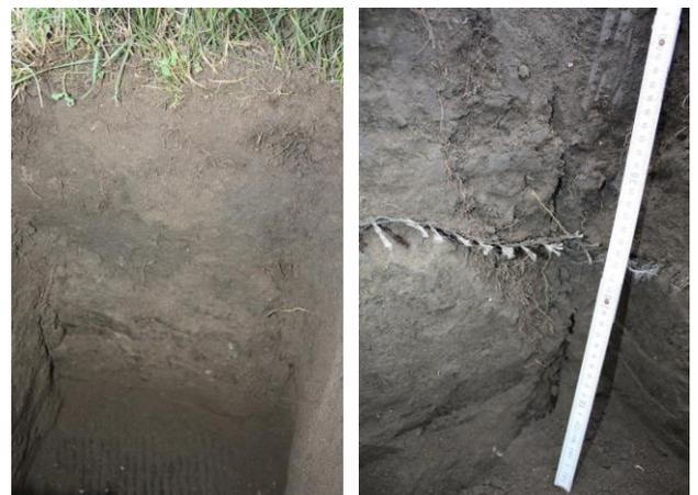
Figure All.59. Material M1 soil horizon depth 60 cm (3D-RM) (l), Material M2 3D-RM in 30 cm depth (visible rooting and cracking) (r)
