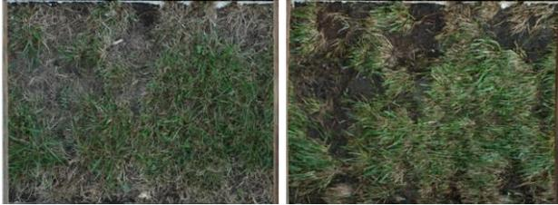
Figure All.55. Cross section E (52 x 38 cm) with erosion mat, flume 1, section 6, initial situation (l) after the fourth test (r)
