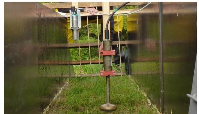
Figure All.17. Ultrasonic sensor to measure runoff depth (left), magnetic-inductive sensor to measure flow velocity (right)
