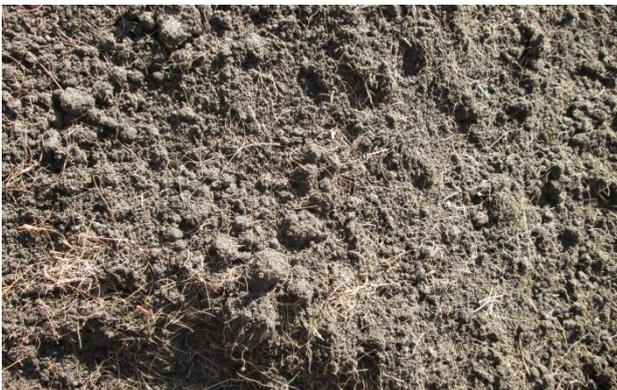
Figure All.142. Good fibre distribution in the DM
