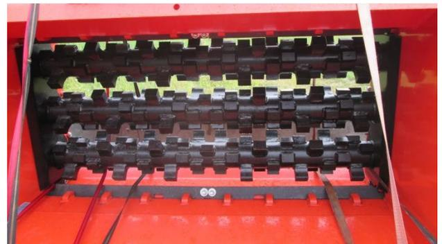
Figure All.138. Drum with blades of the screener crusher
