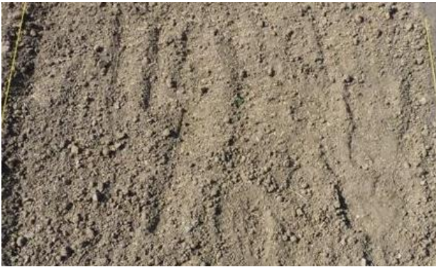
Figure A1.15. Seed bed preparation in the DredgDikes project: fine crumbly dredged material on the top layer.
