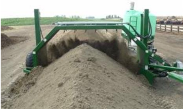
Figure 5.2. Heap piling and homogenisation with windrow turner [15]
