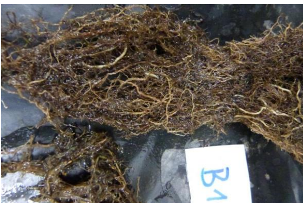
Figure 5.15. Strong root network system (Rostock test dike)
